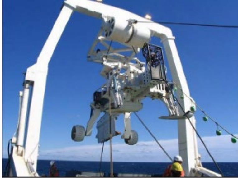
Figure 16. Photo of the IT Plough.
