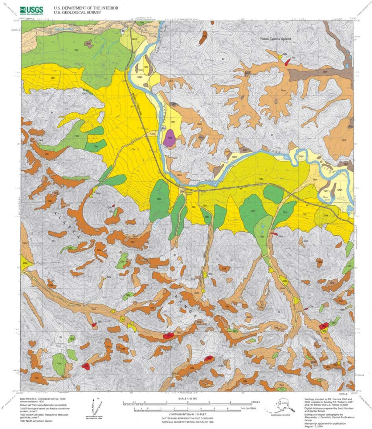
Figure 2.5. Surficial geologic map of the Yerrick Creek Hydroelectric Project area (Carrara, 2004)
