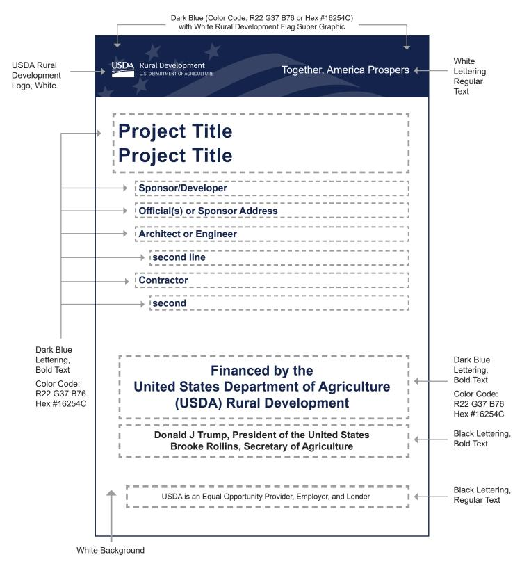
**SIGN DIMENSIONS:** 2400mm x 1200mm x 19mm (approx.8'x 4' x 3/4") PLYWOOD PANEL (APA RATED A+B GRADE-EXTERIOR)
