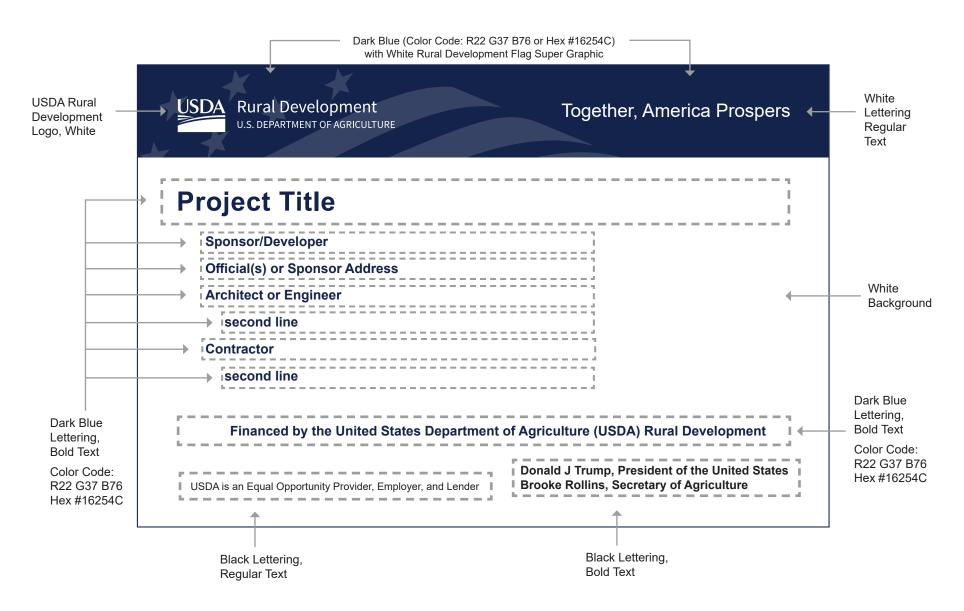
**SIGN DIMENSIONS:** 1200mm x 2400mm x 19mm (approx.4' x 8' x 3/4) PLYWOOD PANEL (APA RATED A+B GRADE-EXTERIOR)
