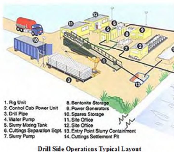
Figure 6-1: Typical HDD Drill Side Work Space
