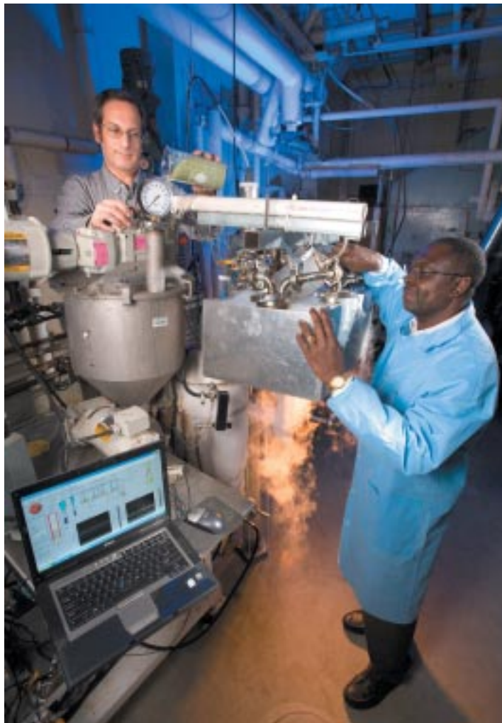
Engineers Neil Goldberg (left) and Akwasi Boateng operate a thermo-chemical reactor they designed and built for converting crop residues into renewable bio-oils and fuels. Top: Elite bioenergy switchgrass in eastern Nebraska. USDA/ARS photos
