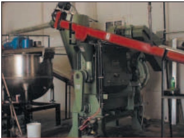
A small, relatively inexpensive crushing press and grease kettle can be set up on farms to produce bio-based greases for use at the site or for sale. Photo courtesy ABIL
